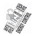
AWARNING Always perform the Lockout / Tagout Procedure before removing any sheet metal panels or attempting to service this equipment.
